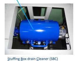
Effectively clean the stuffing box drain pipe and separate solid sludge in settling pan.
